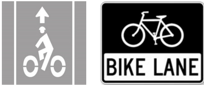
Figure 38: Bike Lane Pavement Marking & Bike Lane Signage
