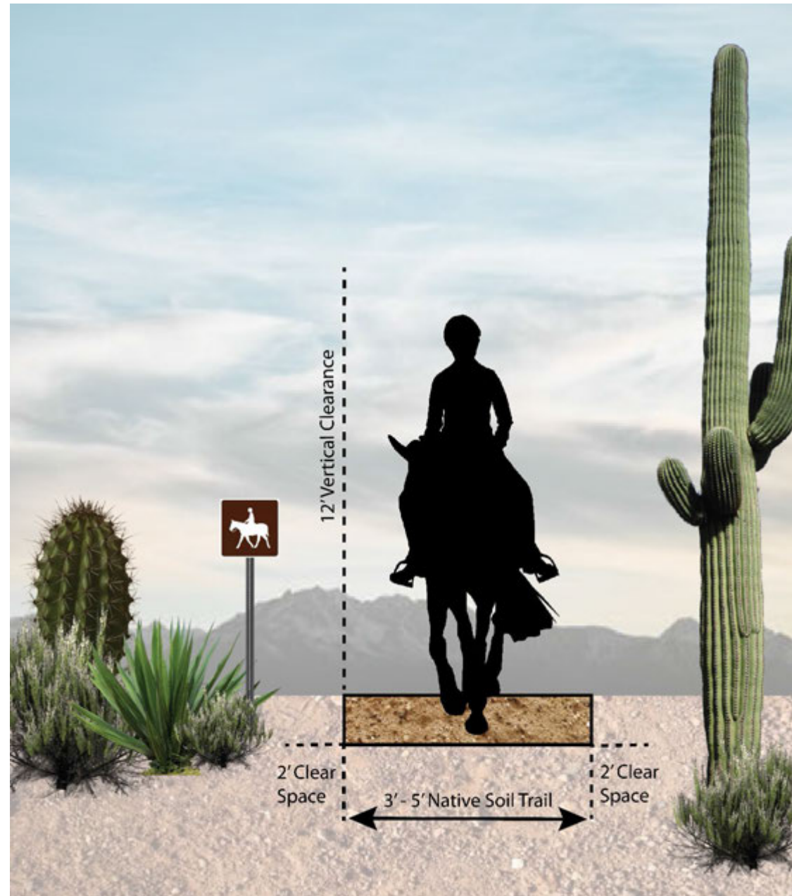
Figure 53: Native Trail Cross Section
